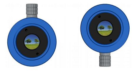
As soon as a parallactic mount or a star diagonal comes into play, the horizontal position in the eyepiece may not be so easy to see. A simple method is now e.g. to find the direction of the dispersion by looking into the eyepiece when the ADC is in neutral position (click position).
