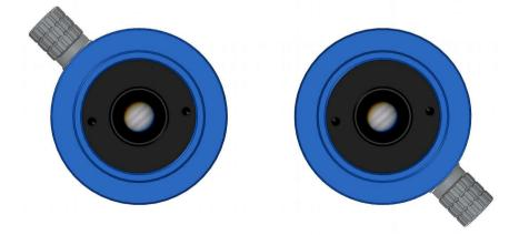
This is relatively easy to see with low standing objects. Now turn the prism unit around the optical axis, so that the adjusting wheel points again in the direction of the dispersion. Again it does not matter if the adjusting wheel (in relation to the eyepiece view) points in the direction of zenith or nadir.
